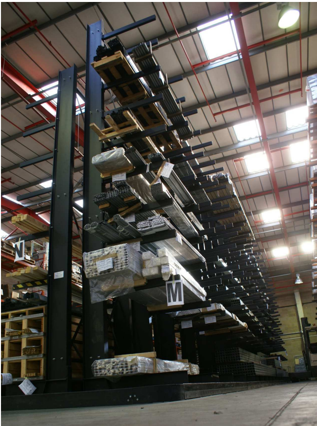
Cantilever racking in new HQ warehouse
